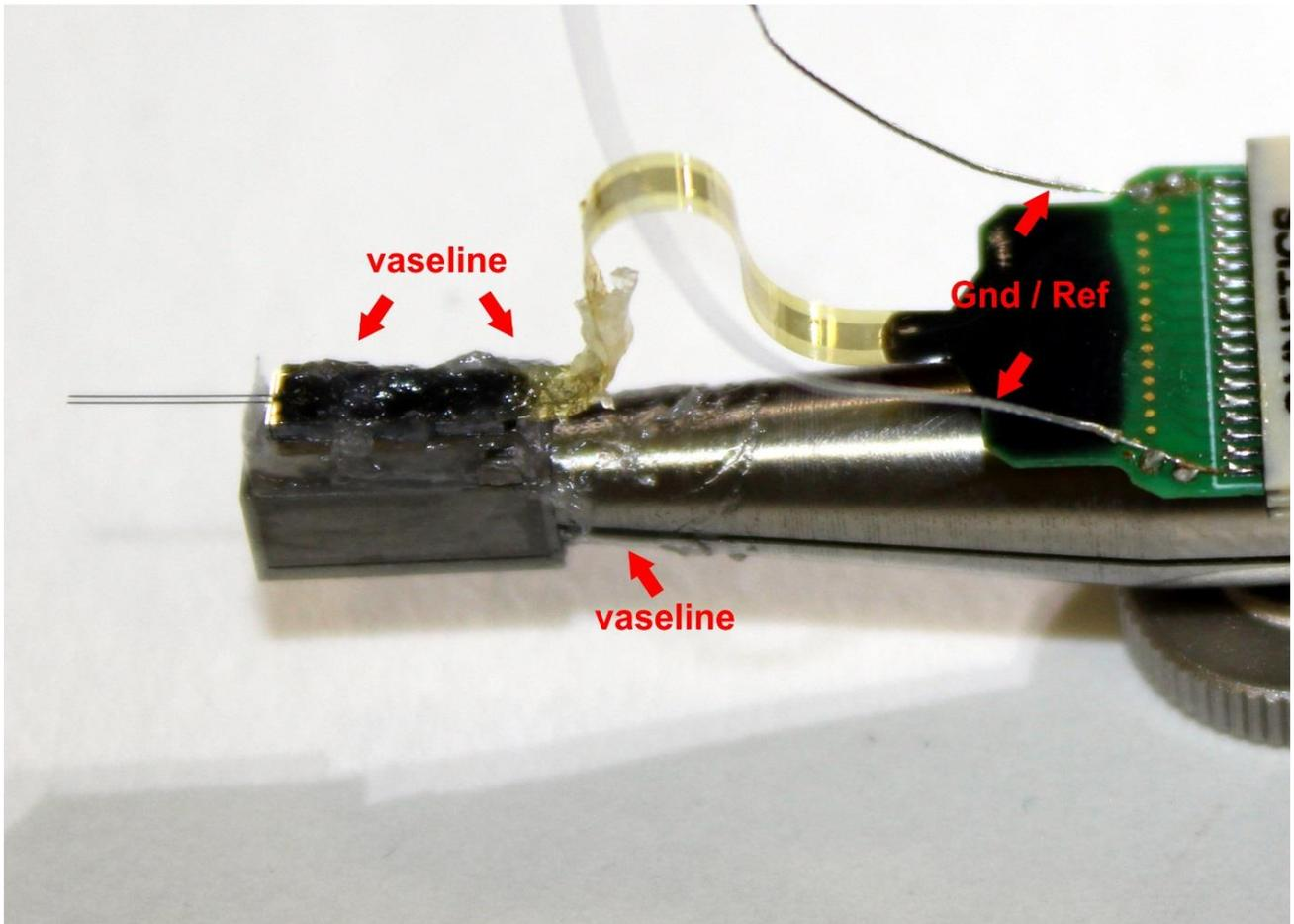
1.6 Prior to implantation, wash and sterilize the probe with 70% ethanol and allow to air-dry.
