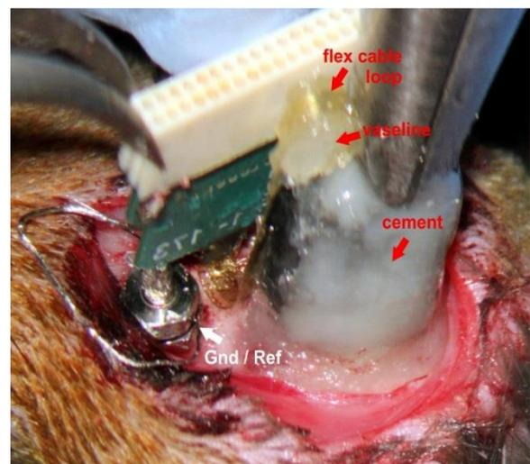
2.11 Cover the probe flex cable loop with cement and build the
