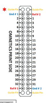
Red Wire and White Wire correspond to indicated REF and GND pins on the probe connector - verify how these connect to your headstage pre-amplifier (1 wire may be sufficient if you prefer GND / REF shorted-together in your headstage).
