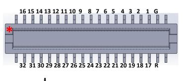
Electrodes are located on the side of the probe as indicated by the arrow below - use Shank A orientation as a reference to construct the channelmap in to your headstage pre-amplifier.
