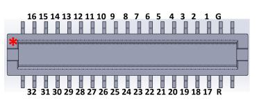
Electrodes are located on the side of the probe as indicated by the arrow below - use Shank A orientation as a reference to construct the channelmap in to your headstage pre-amplifier.
