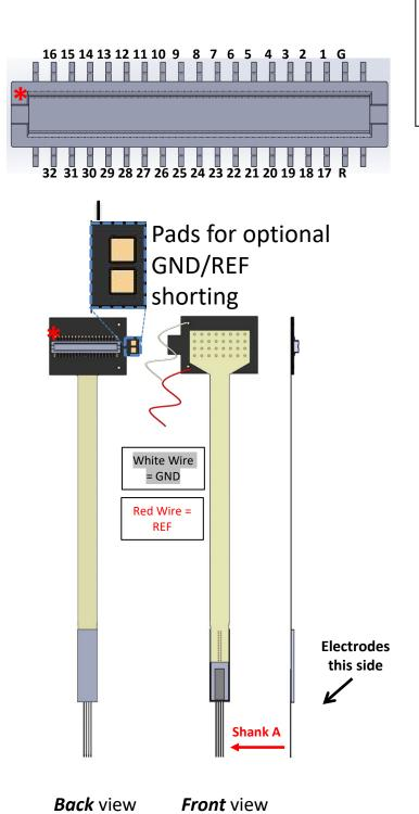
Electrodes are located on the side of the probe as indicated by the arrow below - use Shank A orientation as a reference to construct the channelmap in to your headstage pre-amplifier.
